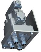
Mounted in the operators preferred position directly to the host machine. Externally mounted 2 Way Valves takes the one way flow from your hammer circuit and then utilizing an electrical switch (runs back to the cab) allow for easy forward and reverse control of the drive unit.
